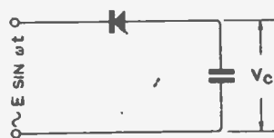
Fig. 7.—Connections of apparatus with which the values of E_c on open circuit for various signal voltages were measured.
