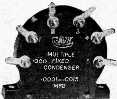
C.A.V. receiving circuit condenser with which capacity values between 0.0001 and 0.0015 mfd. can be obtained in steps of 0.0001 mfd.
