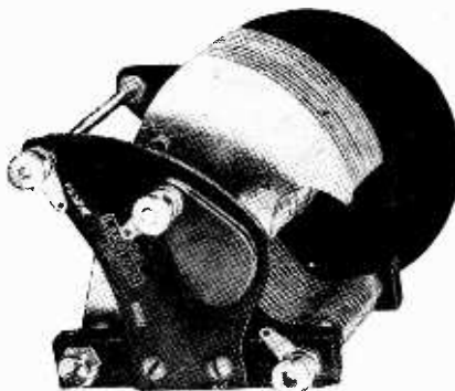
The Lamplugh condenser is fitted with ball bearings and the plates are of somewhat unusual design. The fibre cover to be seen on the metal end-plate protects the bronze spiral, which connects to the moving plates.
