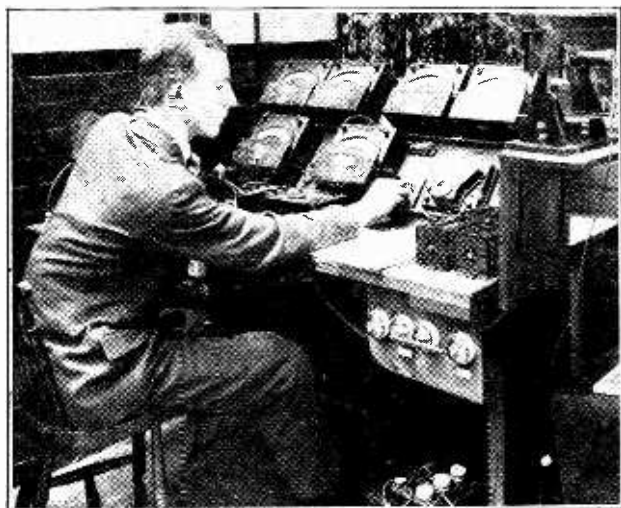
Fig. 19.—A proportion of the valves at the Burndept valve factory are taken each day and carefully checked on this testing outfit.
