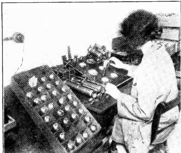
Fig. 18.—Testing valves at the Mullard Factory.
